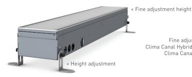
Fine adjustment height (max 0.8 cm) Clima Canal Hybrid: min 10 cm > max 10.8 cm Clima Canal: min 8.5 cm > max 9.3 cm
